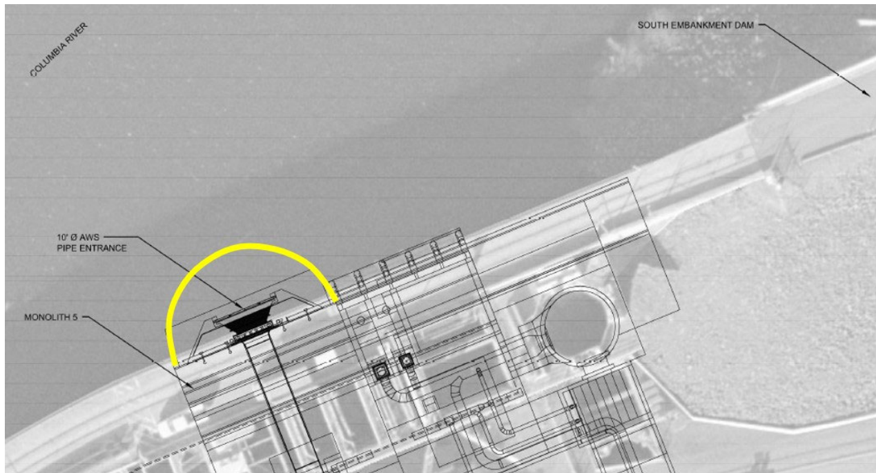
Plan view of existing entrance to AWSBS with triangular and semicircular floating boom or floatingcurtain
